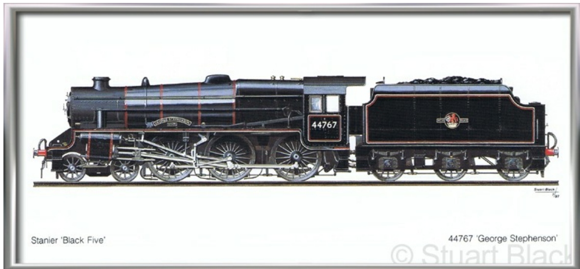
The Class 5 locomotive 44767 "George Stephenson" fitted with Stephenson's valve gear driven from two return cranks on the end of the crank axle rather than two eccentrics.
