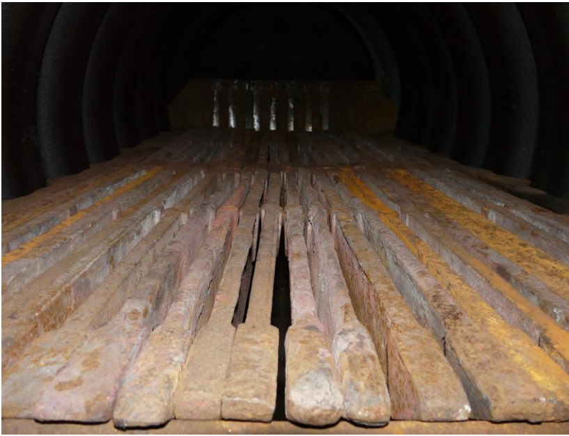
The clean cast iron fire bars of Lydia Eva
